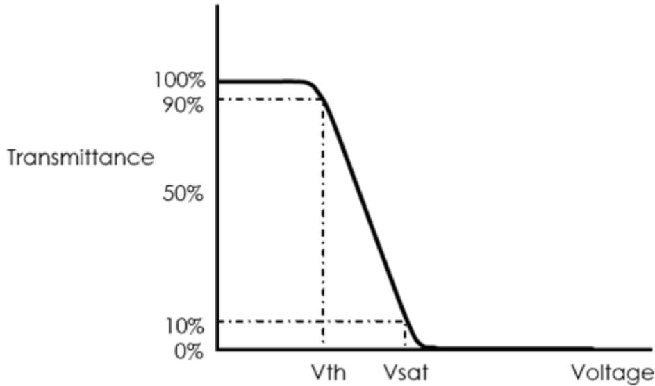
**Figure 2. The definition of  $V_{th}$  &  $V_{sat}$**
