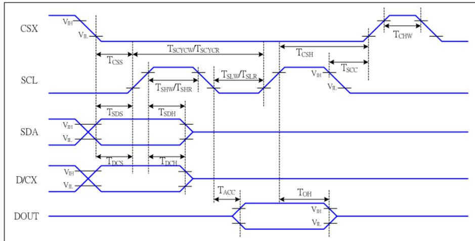
Figure:4-line serial Interface Timing Characteristics
