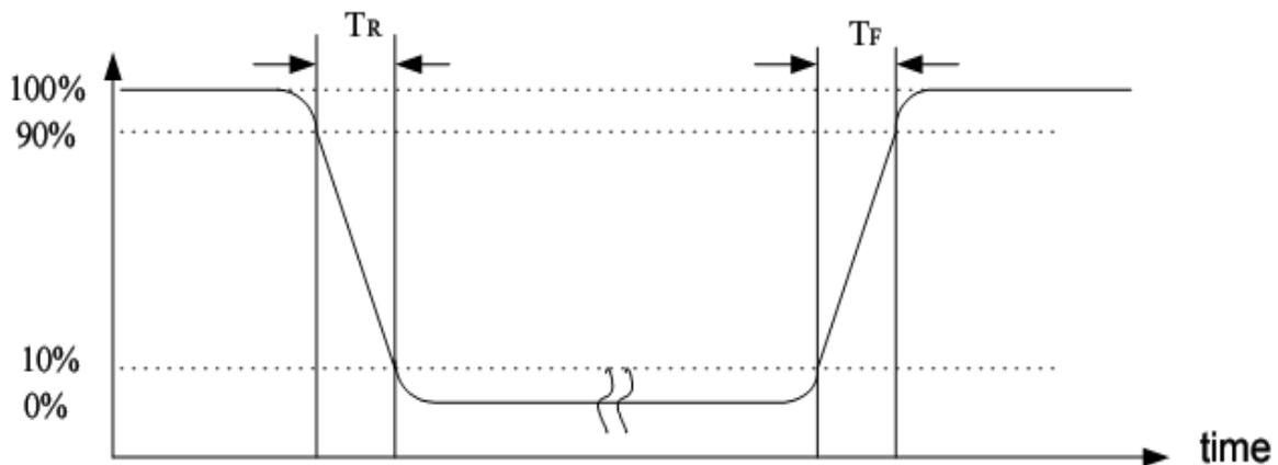
**Figure 9. Definition of response time:  $T_r + T_f$**
