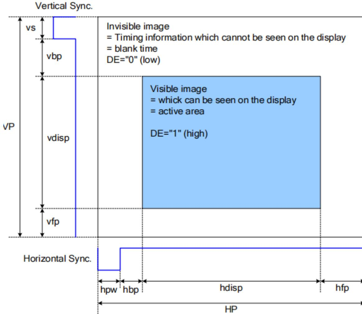
Figure 4 Access Area by RGB Interface
