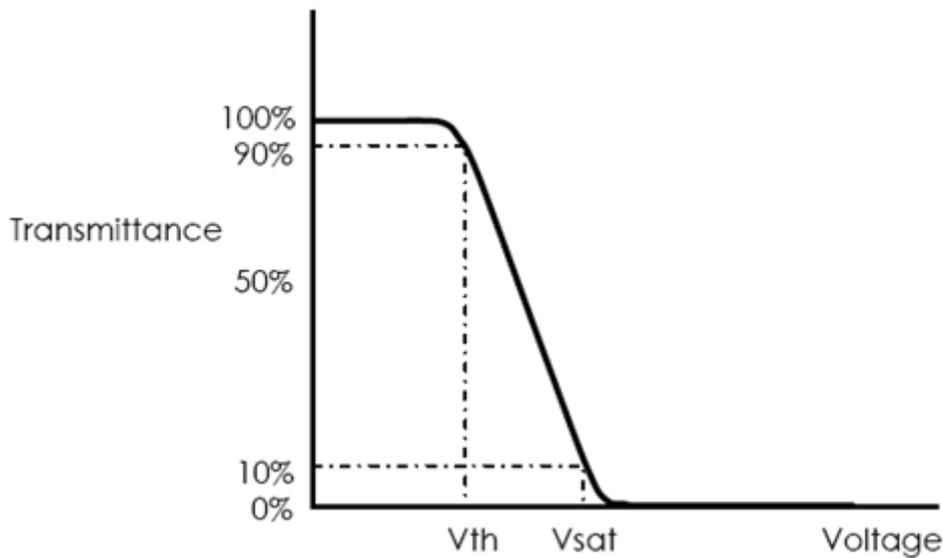
**Figure 2. The definition of  $V_{th}$  &  $V_{sat}$**
