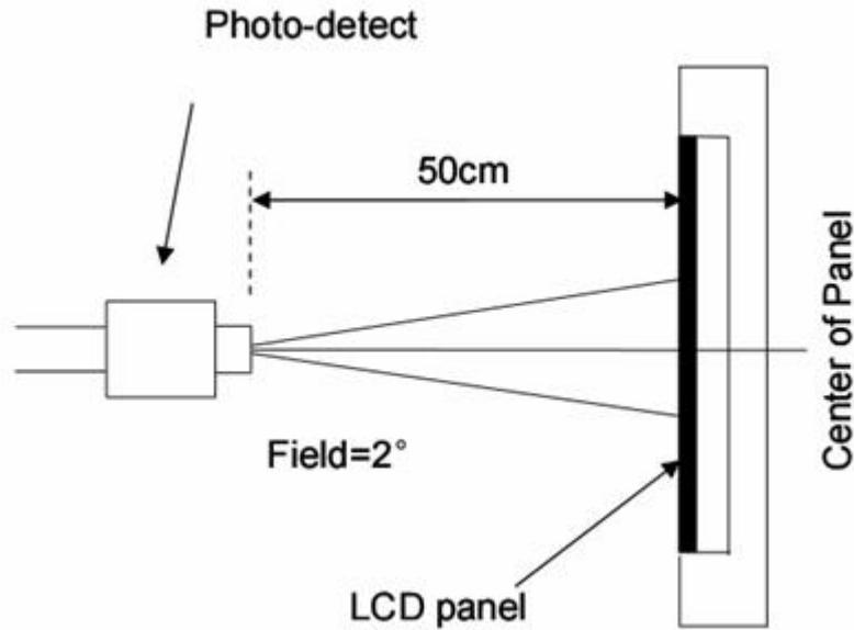
**Figure 4 Optical test equipment.**
