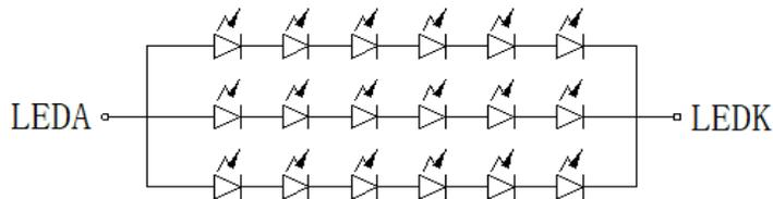
$$I_f = 20 * 3\text{mA} , V_f = 18 \pm 1.2\text{V}$$
