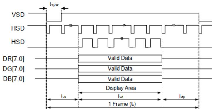
Figure : 24-bit parallel RGB mode horizontal/vertical input timing
